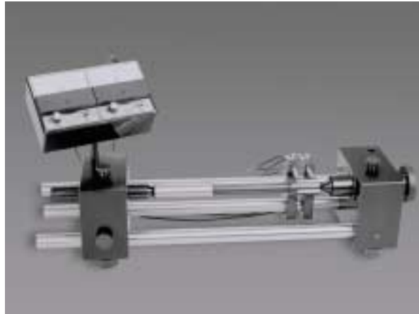
All-purpose setting fixture with electronic indicators
