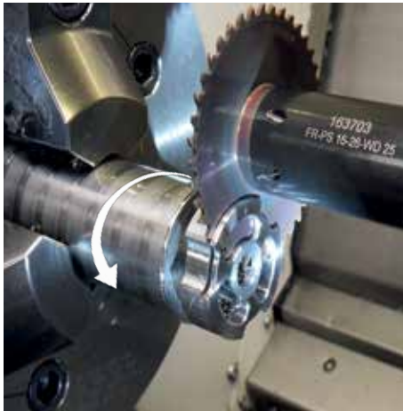
Cutting of VA structured components Vc = 160 m/min Fz = 0,1 mm
