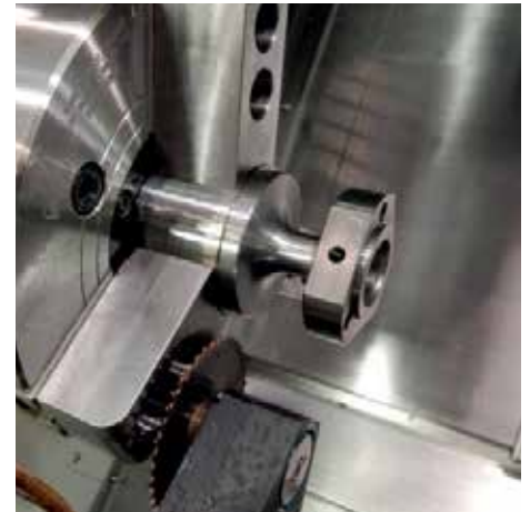
Turn Cut Milling: aluminium Vc = 800 m/min feed = 7m / min
