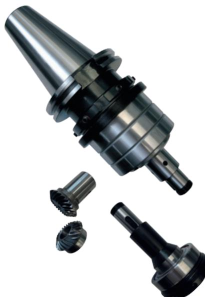
Tools with internal coolant through the spindle (i.C.): To avoid premature wear and damage to the seal system we recommend to filter the coolant to  $40 \mu m$  minimum. Filter grades of  $40 \mu m$  worked in operation with very good results. The maximum permissible coolant pressure can be taken from the technical data of the driven toolholder.
