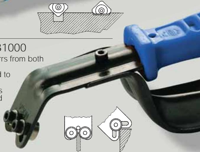
All blades are made of H.S.S.. Hardness 62-64Rc except N80M42 and N80KM42, 65-67Rc.
